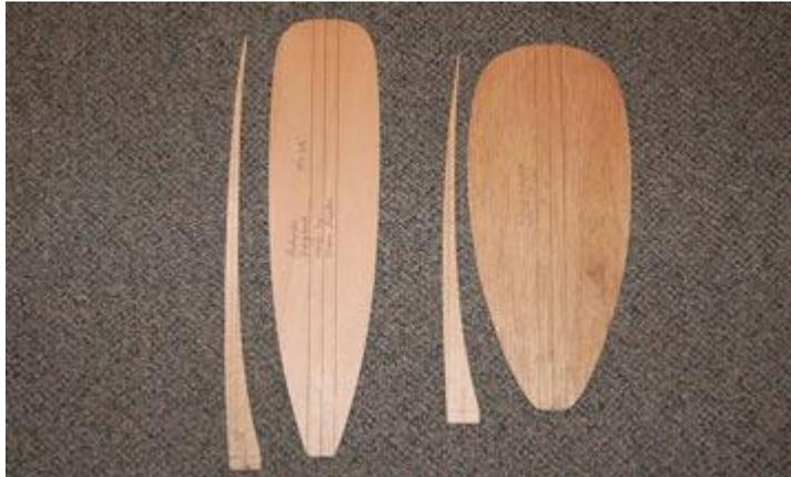
**Blade curve and blade templates made of thin plywood. Note the guidelines.**
