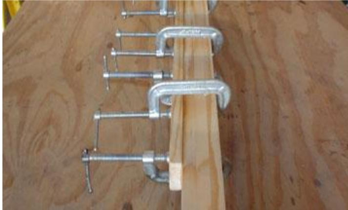
**Laminating a piece of wood to the shaft in the blade area while it is still square allows for a deep curve where the blade is epoxied on.**
