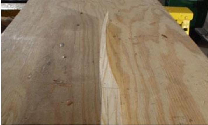
**The curved section cut out of the shaft where the blade will be epoxied on.**
