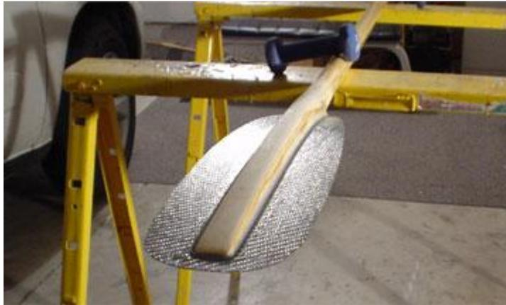
**The back side of a blade after being epoxied to the shaft.**
