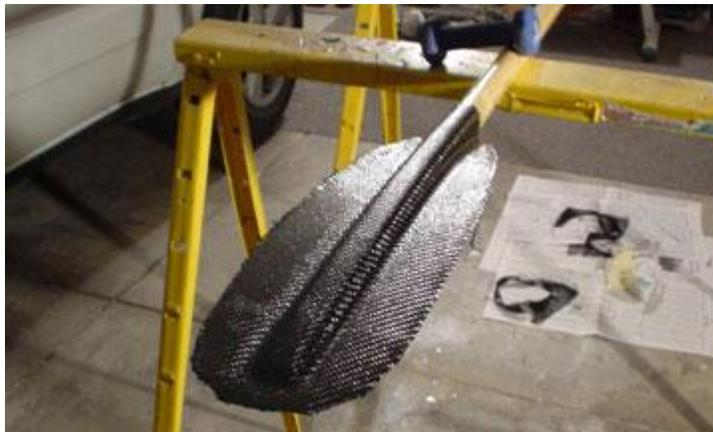
**The back of the blade after the tip reinforcement and a layer of carbon fiber have been added.**
