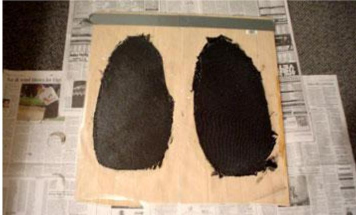
**The blade lay-up is wetted out with epoxy resin.**
