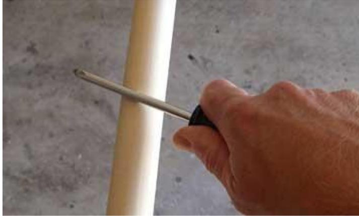
**Hardening the shaft with the side of a screw driver to make it more resistant to denting.**
